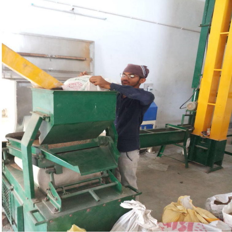
Cleaning and destoning
